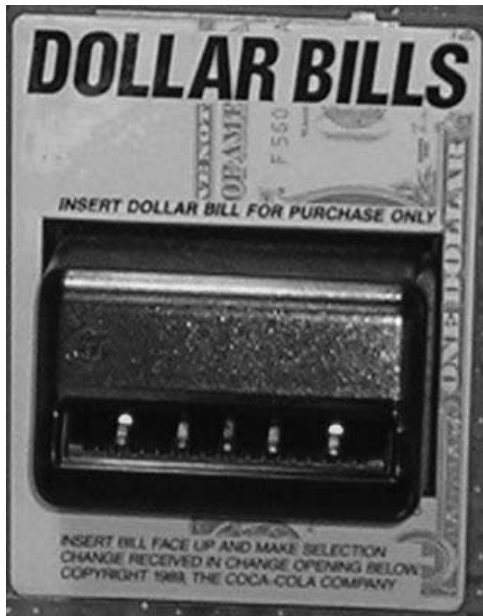
Figure 2: A sign on the Coke machine suggests that bills should be placed into the slot in the lefthand orientation.
