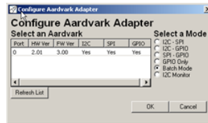
Figure 8: Configure Aardvark Adapter Window The Configure window is organized in two major sections: the list of available Aardvark adapters and the list of operational modes.
